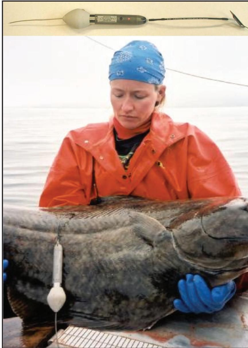
**Figure 1. *Upper panel:* A PAT tag bearing the leader and dart assembly. The tag body possesses sensors that record temperature, depth, and light, as well as a release mechanism that jettisons the body from the leader on a pre-programmed date. The tag then floats to the surface and broadcasts the accumulated data to passing satellites, which in turn use the tag's signal to calculate its position. *Lower panel:* An IPHC sampler holds a large halibut bearing a PAT tag.**
